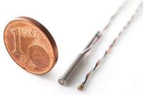
Figure 1 - Sensorade miniaturized pressure sensor
